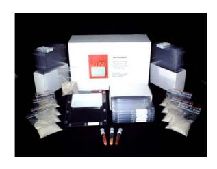
Each Phytotoxkit contains all the materials to perform a complete test with one monocotyl and two dicotyl plant species, in 3 replicates
