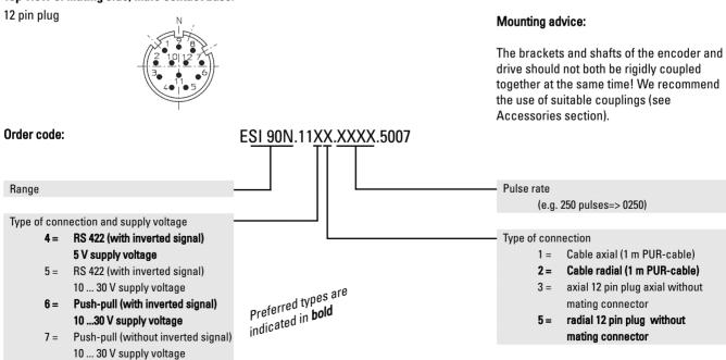
Sensor cables are connected to the supply voltage internally if long feeder cables are involved they can be used to adjust or control the voltage at the encoder
