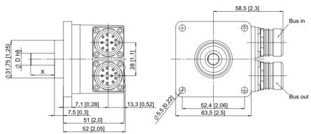
ø 58 mm, Clamping flange Flange type 1 and 3 (Drawing with 1 x M12 connector)
