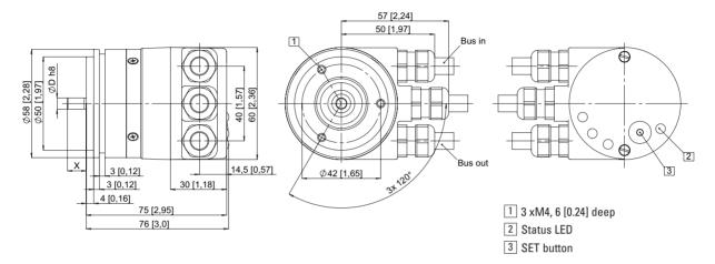
ø 58 mm, Clamping flange Flange type 1 and 3 (Drawing with 2 x M12 connector)
