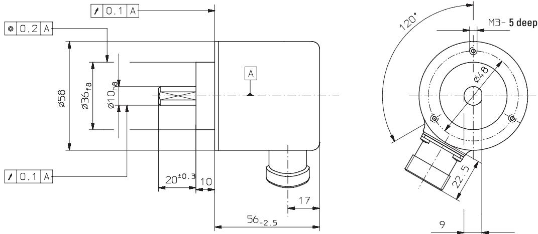
Synchronous bracket with shaft ø 6 mm
